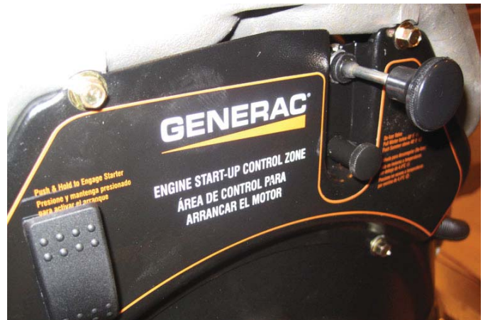
Figure 19 - Full Choke Position
