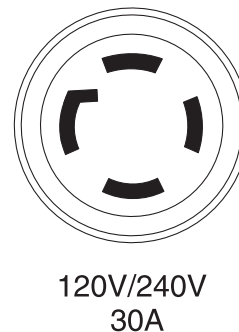
Figure 12 - 120/240 VAC, 30 Amp Receptacle
